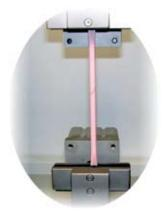
When the sample breaks it is often at the joint area. This does not infer weakness but at such high elongation, a surface imperfection around the joint area will be the point of breakage.
